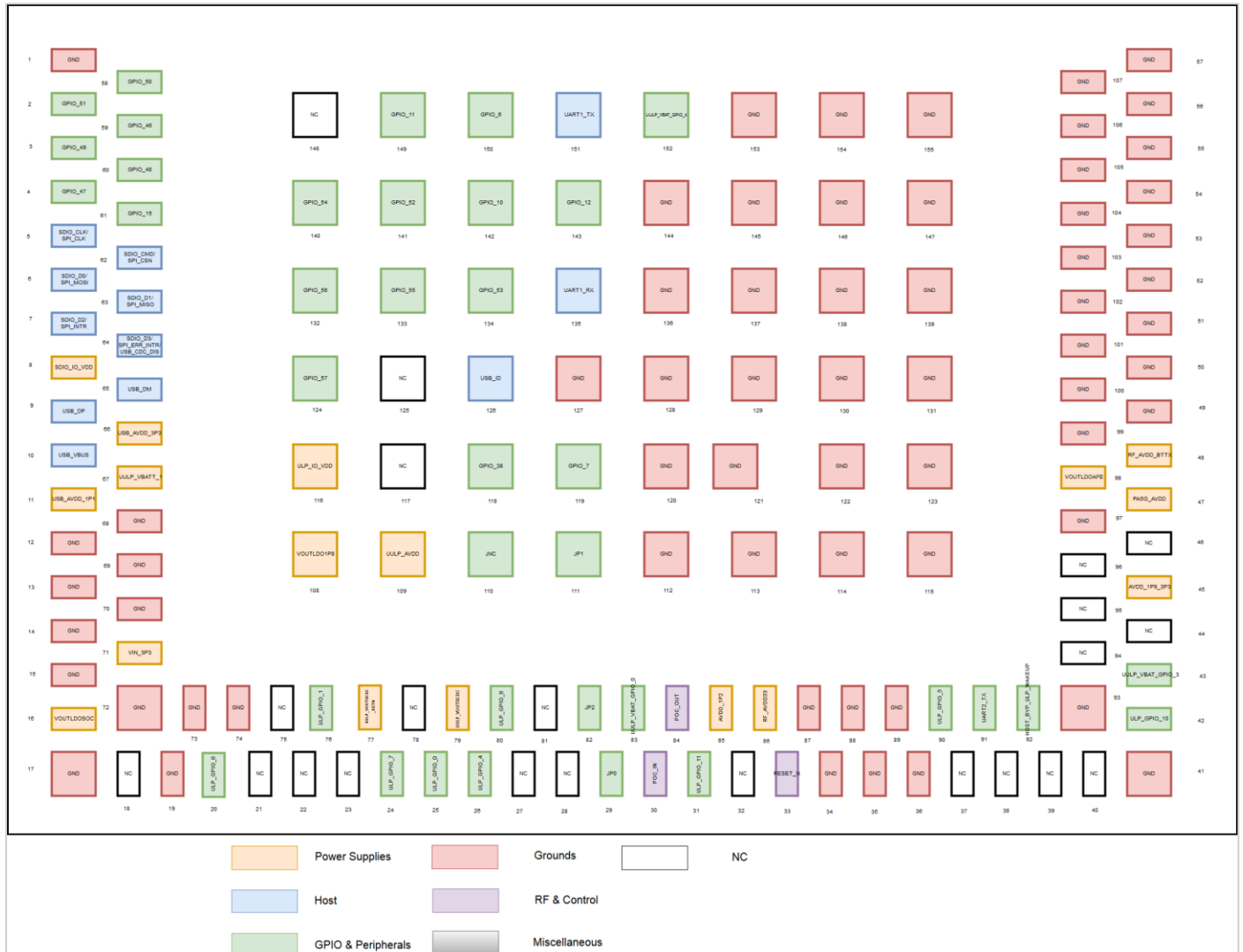
Figure 5. RS9116 CC1 Pin Diagram
